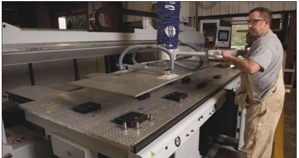
All four major pieces of CNC equipment at Giffin Interior & Fixture are integrated in to the company's lean concept and are linked. A key piece of equipment is a Homag BOF611 CNC machining center with Flex 5 Aggregate. The BOF, purchased through Stiles Machinery, is the centerpiece of the company's nested base manufacturing process within the component production work cell. The BOF utilizes barcoding to set up the machine and track orders and parts. Machine linkage within the entire plant is accomplished using a number of software packages, including Pattern Systems, Cutrite, Woodwop and Holzlink.
