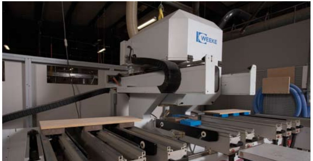
A Weeke BP12 machining center utilizes barcoding technology to track orders and parts and set up the machine.
